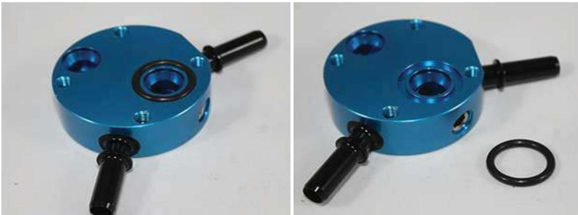
7. Install the new supplied O-rings on both the Stage 2+ pump as well as your new Stage 3+ pump. As shown in step 16 of the Stage 2+ assembly instructions.
