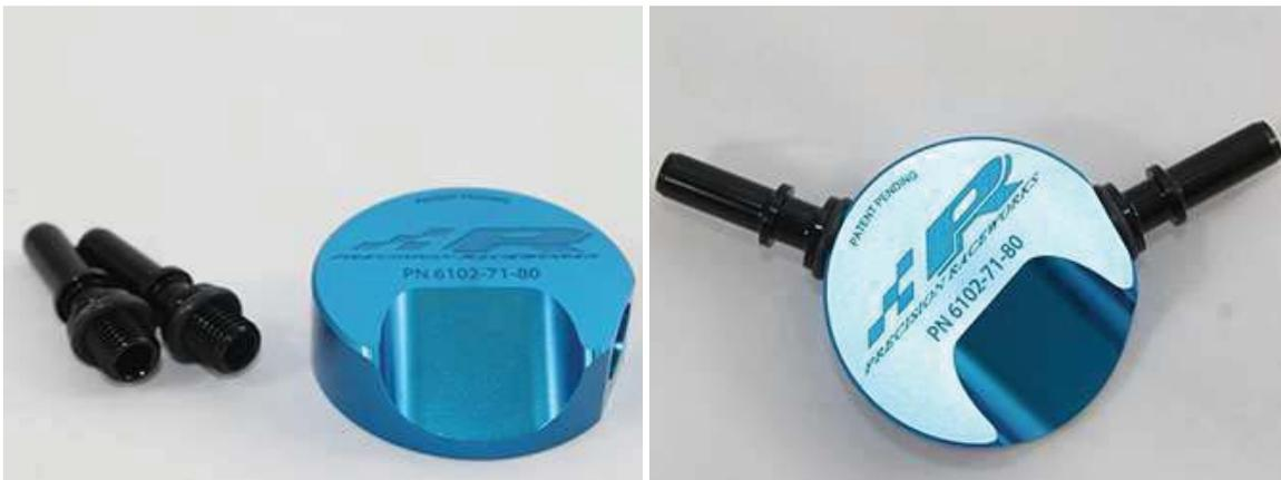
15. For the O-ring to go into the fitting you will no longer be able to tighten by hand as it is a very tight fit for a perfect seal. For final tightening we recommend using a **leather work glove** to protect the finish on the fitting and a pair of pliers to tighten. Tighten the fittings until close to flush with the OD of the part.
