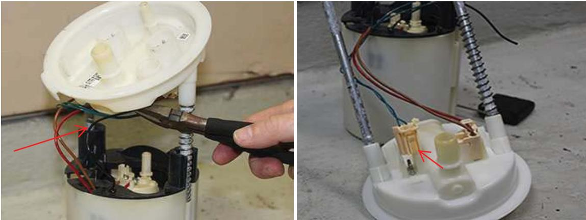
3. Remove the fuel float assembly by pushing back the two tabs shown in the photo below. While pushing in these two locking tabs lift up on the fuel float assembly to remove it.
