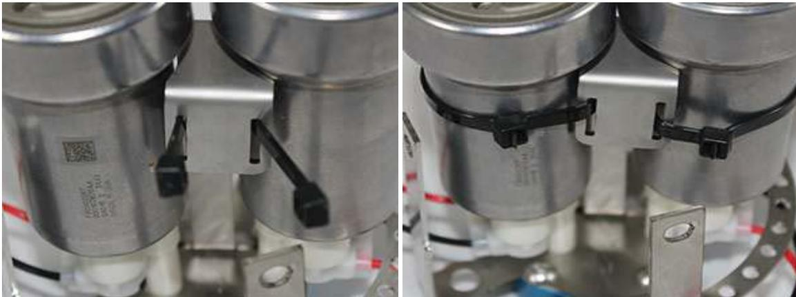
11. Run the wiring through the required holes in the 3 leg bracket and remove the nylon wire grommet from the Stage 2+ bracket and install along with the new grommet as shown in step XXX of the Stage 2+ assembly instructions.
