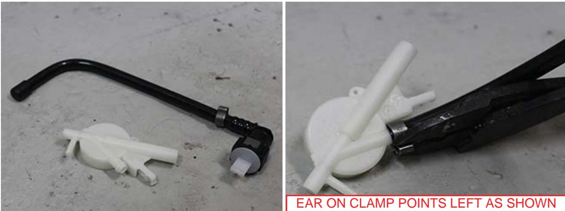
11. To install the venturi drill 4 holes in the bottom of the fuel bucket using your small drill bit and working up to one large enough for the supplied nylon zip ties to pass through the holes. The holes do not have to be on an EXACT location but the images below and use of a flashlight can help better understand where to drill the holes.
